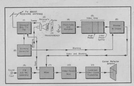
Fig. 2. Block diagram of transmission system showing functions of the units.
