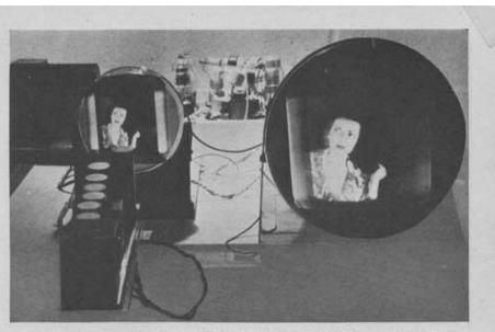
Fig. 6. The original transparency (left) compared to the reproduced image (right).
