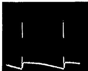
14. Terminal 6 of vertical oscillator transformer, V.O.S.T., 7 volts, p/p, 60 cps.
