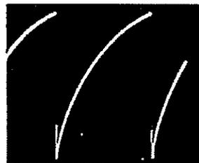
15. Vertical oscillator base, 3.5 volts, p/p, 60 cps.
