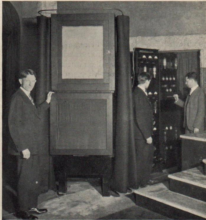
One form of receiving apparatus for television; the distant scene is made visible to the audience on the glass screen in the center of the picture. Dr. Frank Gray, who is largely responsible for that method of receiving, stands at the left, his hand resting on a lower screen behind which is the loud-speaking telephone. On the right, W. S. Bishop and E. Peterson manipulate the controls of the amplifier and other associated equipment
