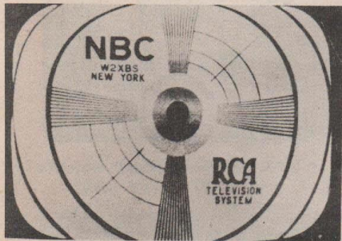
Fig. 9-Vertical Linearity Control Incorrectly Set
