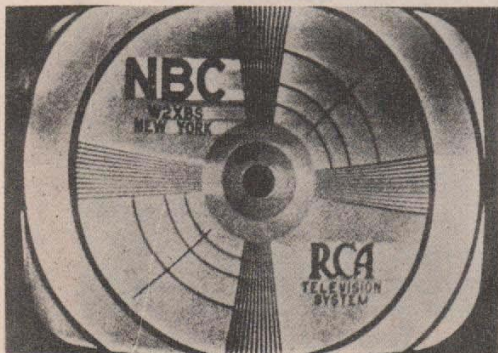
Fig. 13-Phase Shift and Loss of Low Video Frequencies
