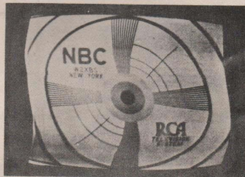
Fig. 12-Excessive Ripple in Horizontal Deflection
