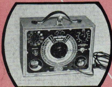
You will use this condenser analyzer to check radio and television components.
