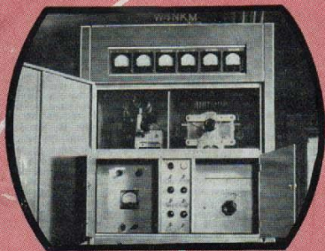
Thousand watt transmitter, for gaining a actual transmitting experience.
