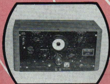
Special signal generator used in aligning television receivers.
