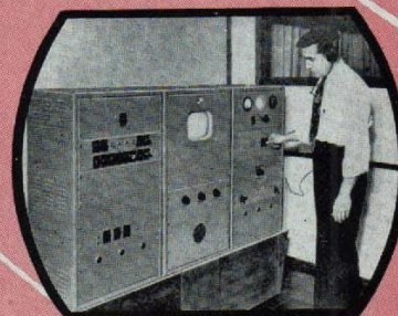
Technician adjusting television camera control equipment.
